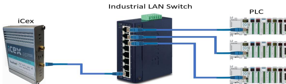
Fig. 2 Connecting multiple devices (PLC) to iCex via Ethernet Switch
