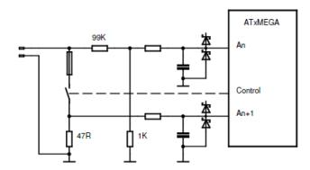
Analog input A/D is 11 bits. The whole range is 0 - 2047.
