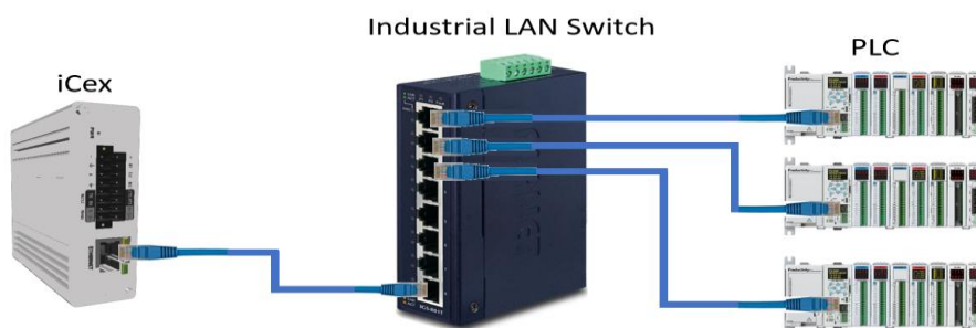
Fig. 2 Connecting multiple devices (PLC) to iCex via Ethernet Switch
