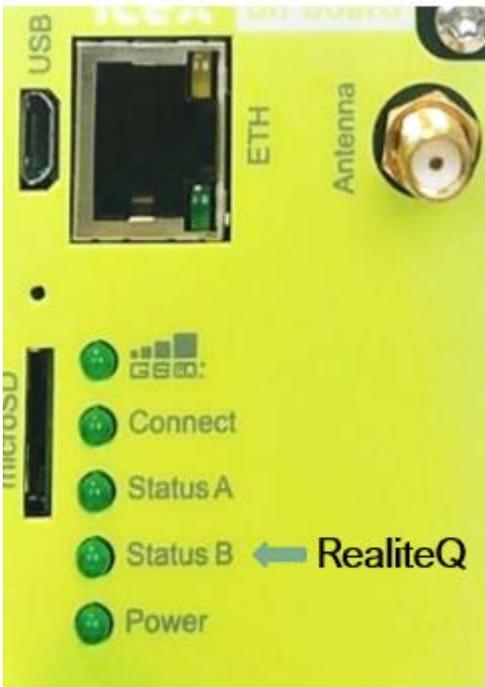
Fourth – **Status B** LED - Starts to blink only after successful connection to Internet (GSM and Connect LEDs are lighting)
