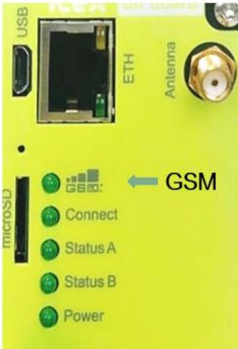
The upper, **GSM** LED is showing connection to provider's GSM network.
