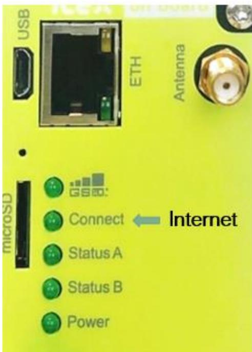
Second – **Connect** LED, is showing connection between Cellular network and Internet. It starts to blink only after successful connection of iCex to GSM network.
