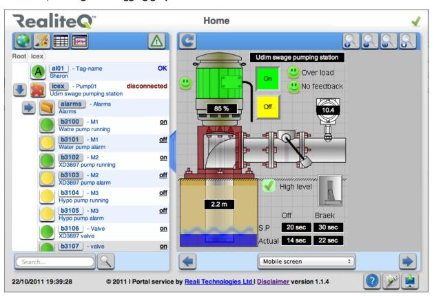
RealiteQ-UI offers a powerful screen engine capable of presenting rich, high-quality graphics to the operator. Graphical elements can be connected to real-time values by means of links. Links can be programmed in a variety of ways to control every aspect of the display, including changing colors, visibility, position, etc. Links can be used to define actions related to mouse operations, such as changing a value, opening windows etc.
