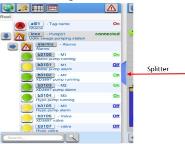
You can control the tree side width by dragging the splitter. You can close/open the window side by clicking on the splitter button.
