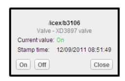
The icon button, path button and value display a textual tooltip when the mouse moves over them. The cursor type and the background color of the pointed button will change too. The tool-tip yellow text window is shown in a delay of one second and disappears after maximum five seconds. The tool-tip window disappears immediately if you click on the button. Moving to point on the tool-tip window area will keep the tool-tip window open.
