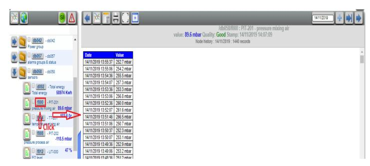
On opening the UI displays the current-day samples log. The data is displaying in descend order - the end date displays on top of the table.
