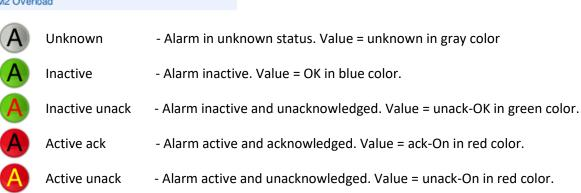
If "alarm has a history" sign appears, clicking on the alarm icon or path will display the alarm history. If the alarm was defined for user acknowledge the alarm value will appear to underline. Click the value will be acknowledges the alarm.
