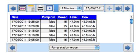
Clicking the table button on the tree toolbar displays the current report log history in the right pane of the screen. On opening the UI displays the current-day log. The data is displaying in descend order - the end date displays on top of the table.
