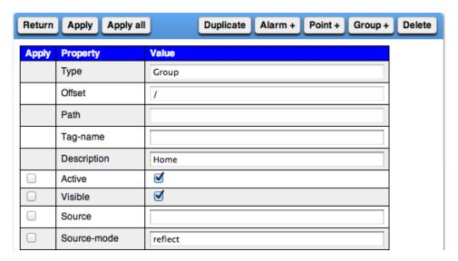
When you edit a group node, you can apply specific fields change to all the group sub-node. The apply button effect only the group itself, by checking the necessary apply check-box and clicking the "apply all" button the setting in the check rows will affect the group and its sub-nodes too.
