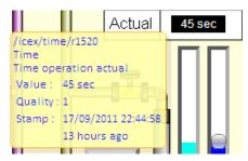
Positioning the mouse over writeable graphical elements will change the mouse cursor to a hand cursor.
