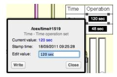
Clicking writeable node value opens write dialog box. The current edit node marks with four black squares. There are two kinds of write dialog window - one for numerical value and one for On/Off set value. The upper part displays the online current node state. The lower part is used to modify the node state value.
