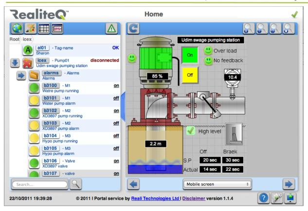
RealiteQ-UI offers a powerful screen engine capable of presenting rich, high-quality graphics to the operator.
